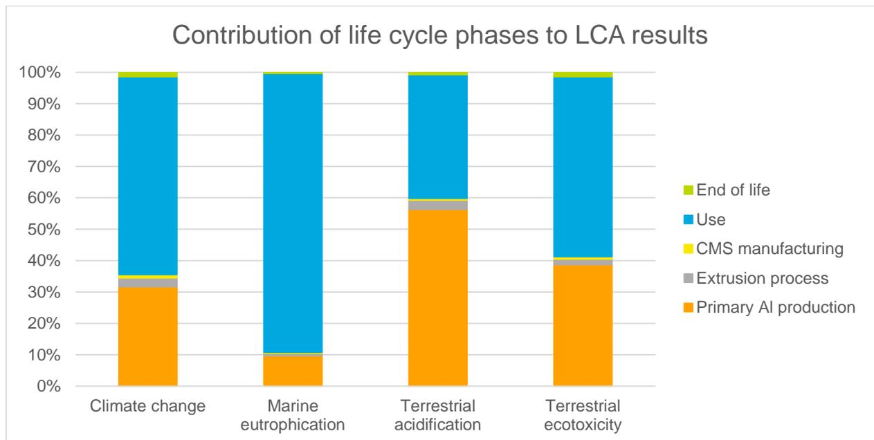
Comparatively to Use and Primary metal production, extrusion process and CMS manufacturing provide limited contributions (1% to 4%) to the overall impacts. This remains true in all considered impact categories.
