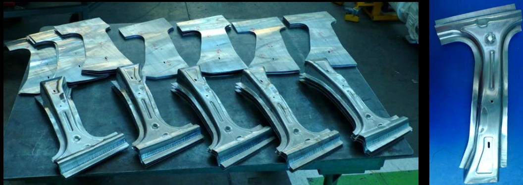
Press-quenched B-pillar reinforcement prototype part (C-TEC internal)
